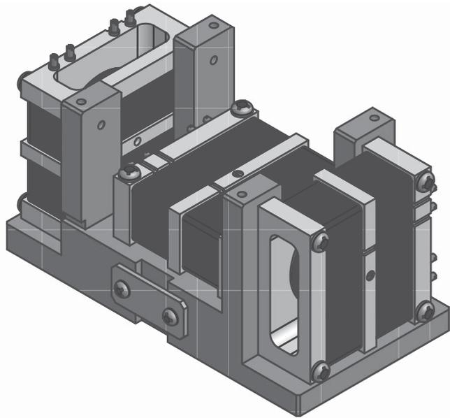
Fig. 4. Tri-axial sensor unit of MGF-IS.
