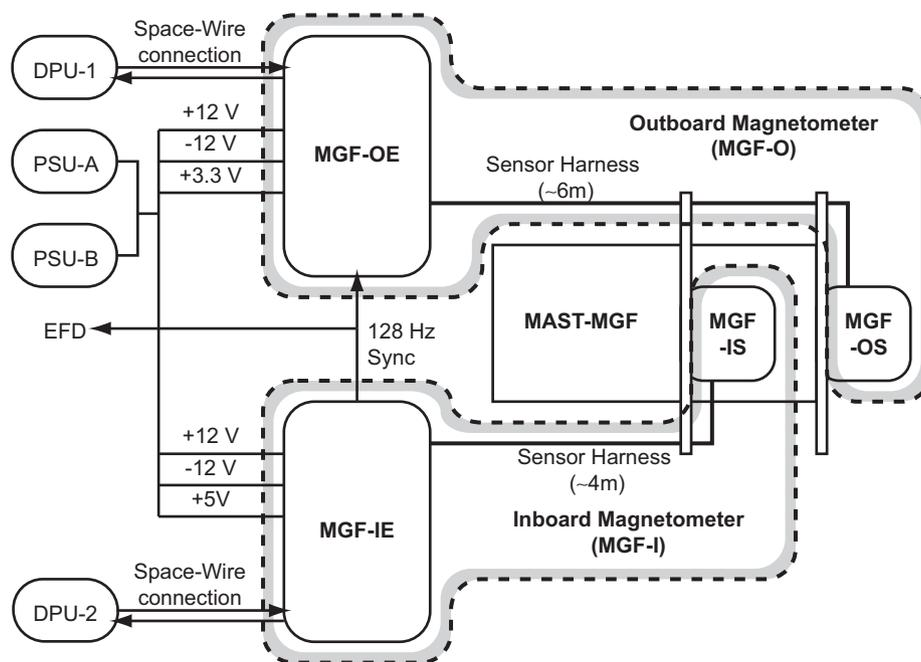
Fig. 1. Block diagram of the MGF magnetometer.
