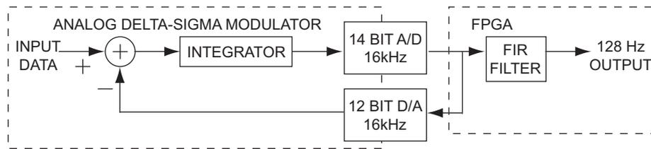
Fig. 6. Block diagram of the delta-sigma analogue-to-digital converter.
