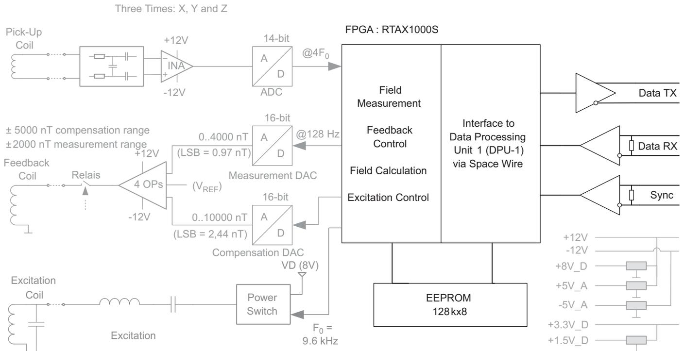
Fig. 3. Block diagram of MGF-O magnetometer.
