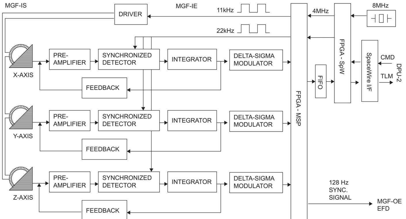
Fig. 5. Block diagram of the MGF-I magnetometer.
